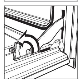
■ Flip up the locking clamps on each door hinge. This locks the hinges.
